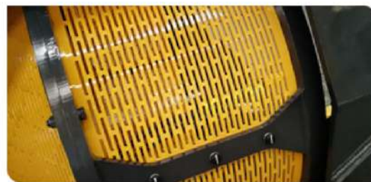
Mesh from 1-120mm, interchangeable
